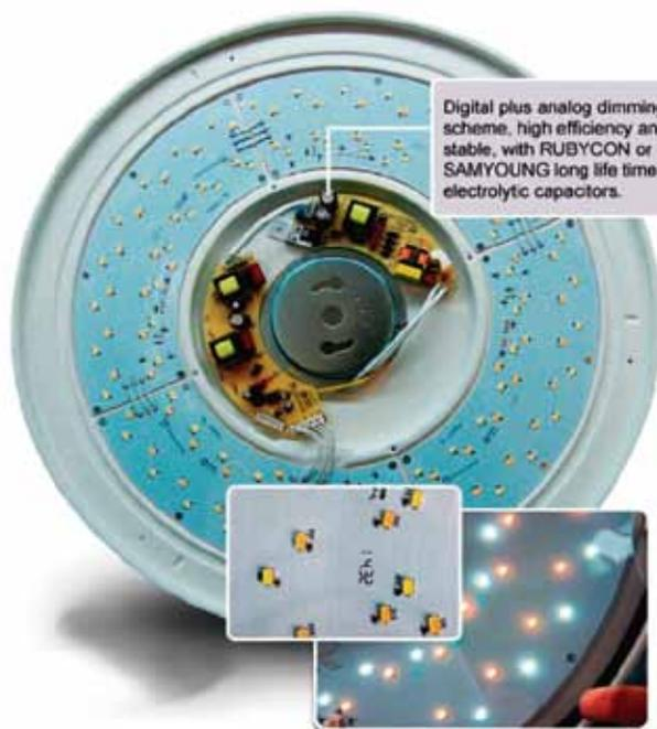
Digital plus analog dimming scheme, high efficiency and stable, with RUBYCON or SAMYOUNG long life time electrolytic capacitors.
